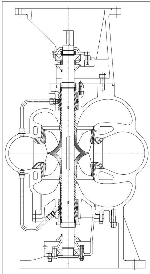
Suction and discharge flanges are located at an angle of 180° to each other. Impeller is double-entry. Shaft seal: packing seal or mechanical seal.
